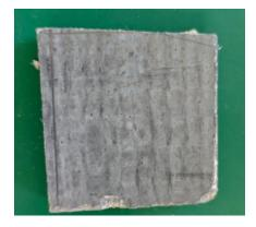
Organic Fibre detected in the reinforcing mesh – note that this is not asbestos, but is included in the report to satisfy NATA reporting requirements
